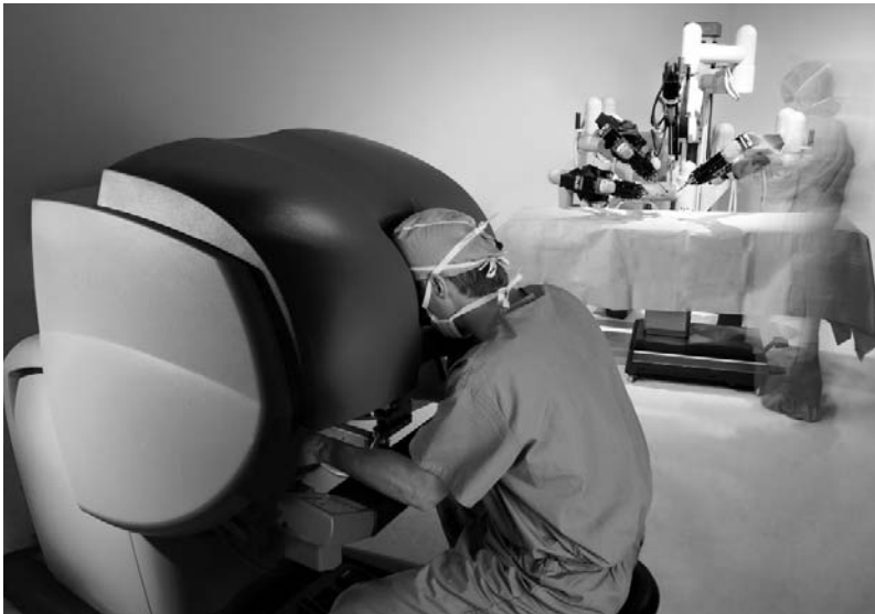
At the robotic console, the surgeon views the operation through a 3-D viewfinder and controls the instruments.
